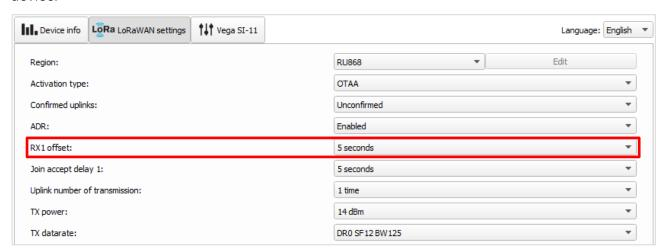
If ABP activation method is used the opening time for the first receiving window must be the same in the device settings in Configurator and on the server.
