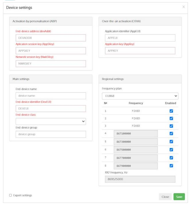
Fig. 2. The main parameters for registering the device on the server.
