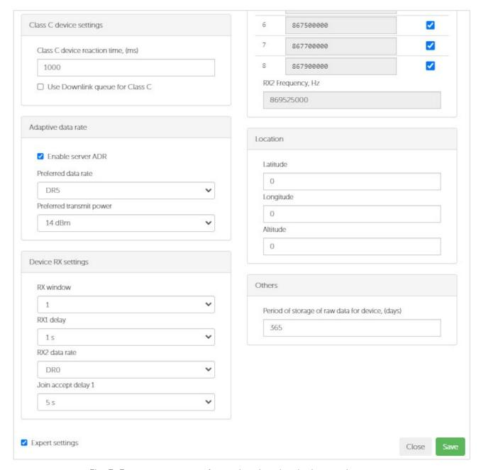
Fig. 3. Expert parameters for registering the device on the server.
